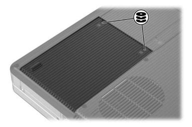
3. To remove the hard drive cover and expose the hard drive tab, lift the cover **①** upward and away from the notebook **②**.
